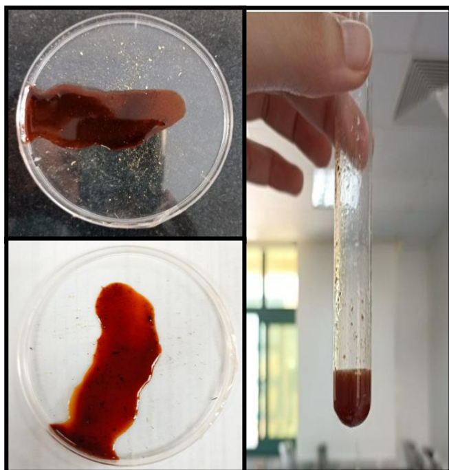
Fig. 3: Qualitative detection of inulin using resorcinol test.
